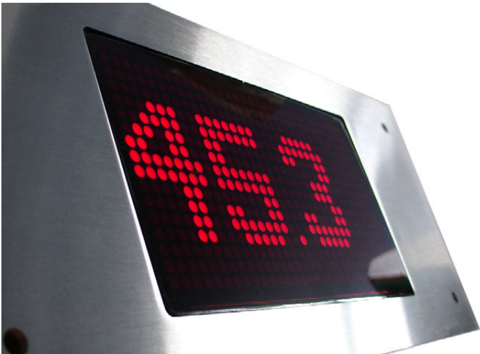
S4-MIO3 has an extra wide dot matrix of 32x16 dots. S4-MIO3 can be fitted to both landscape and portrait, which gives great flexibility for how information is displayed. The display above shows the height above the ground instead of the floor - one of our many tailor-made solutions.
