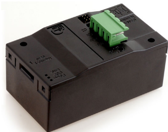
SP02 is a speech processor developed by P DAHL. It has a built-in speaker, SD Memory Card Reader and MP3 player for playback of digital audio files.
